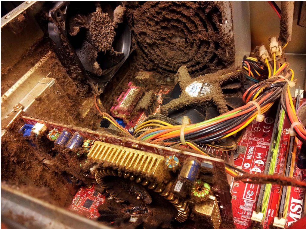
Figure 2. A computer damaged by dust. © Arvutistuudio CC BY-SA 4.0
