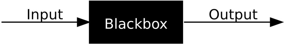
Figure 2. A black box is a device, system or object that can be viewed in terms of its inputs and outputs, without any knowledge of its internal workings. Source: https://en.wikipedia.org/wiki/Black_box
