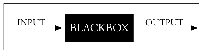
Fig. 1. A blackboxed system processes input into output without the user’s knowledge of the interior functionality of the system. (© Garnet Hertz)
